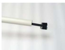
12. Gently push the antenna and cable back into the white tube until it locates into the top of the black tube. (gently pull the cable through the hole drilled in (2) as the antenna is pushed in).
