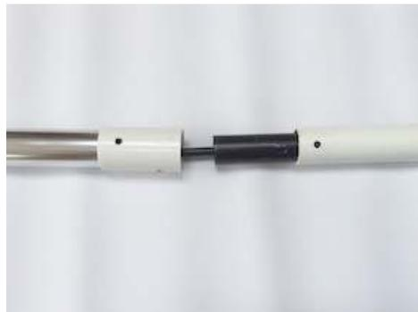
10. Connect the female SMA connector to the antenna end of the coaxial cable (check that there isn't a short between the inner and outer conductors) and attach the P3I antenna.
